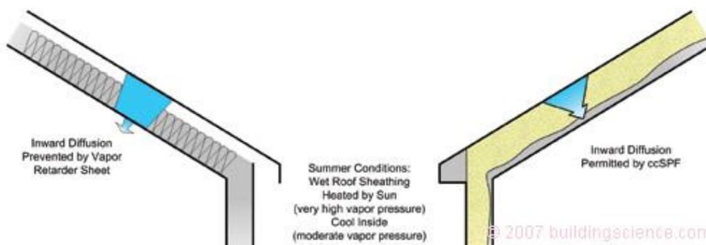
In warmer temperatures, spray foam allows the assembly can still dry to the inside because the spray foam is a vapour retarder rather than a pure vapour barrier.
