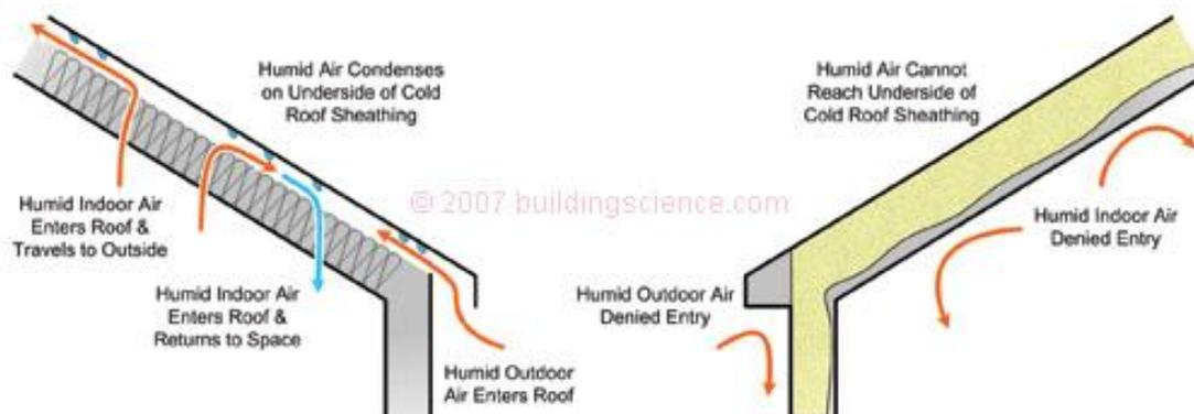
✓ Unvented roof assemblies control heat flow.
