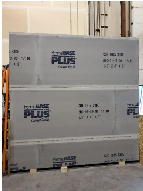
**Figure 4:** The exposed face prior to the stucco application.
