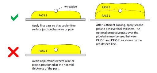
NOTE 1: Some plastic pipe manufacturers prohibit the application of spray foam over certain pipe fittings. The spray foam can be applied to the pipe, but the fittings must not be in direct contact with the foam. The installer needs to check on this prior to spraying foam around any plastic pipes. To avoid chemical contact with fittings, the installer can wrap the fittings in aluminum foil prior to foam application to provide a chemical barrier.
